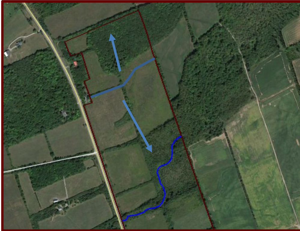
Figure 2-1: Project Site and Drainage Patterns
